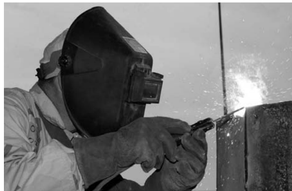
SGT Clay O'Dell, 3-112th Armor Battalion, 56th Brigade Combat Team, 36th Infantry Division, welds a 3/8-inch steel armor plate on a HMMWV in southern Iraq.
