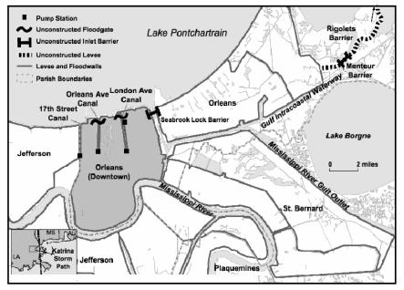
Figure 2. Rejected Inlet Barriers and Canal Floodgates
