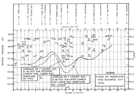
Figure 7. Critical Pressure Derived from Average of Seven Lowest Actually Observed Storms
