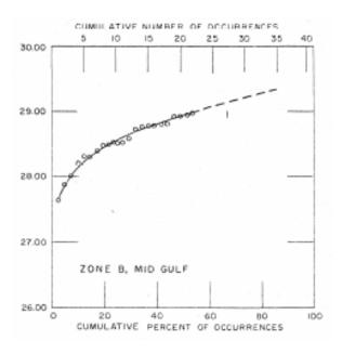
Figure 4. Cumulative Number of Storms in Zone B at Various Pressure Levels, Converted to 100-Year Index
